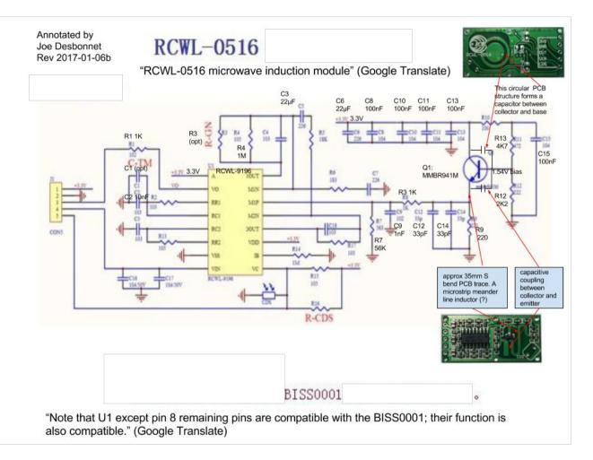
I used spice simulations to verify that small changes to transistor base bias causes changes in oscillation frequency. By running a few simulations I estimate that  $1\mu$ V change in bias will change oscillation frequency by 1.4MHz.
