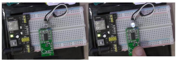
/\*\* Example NOT tested : Log the output pin of a RCWL-0516 radar module to a 433 MHz XY-FST transmitter. \*/
