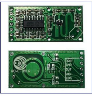
Operating frequency: The product specification omits the operating frequncy. I found a carrier at 3.181GHz on my unit using a HackRF One SDR radio (see spectrum plot below). I suspect this frequency will vary from device to device: it would be difficult to have a tight specification with such a simple RF circuit on FR4 PCB.
